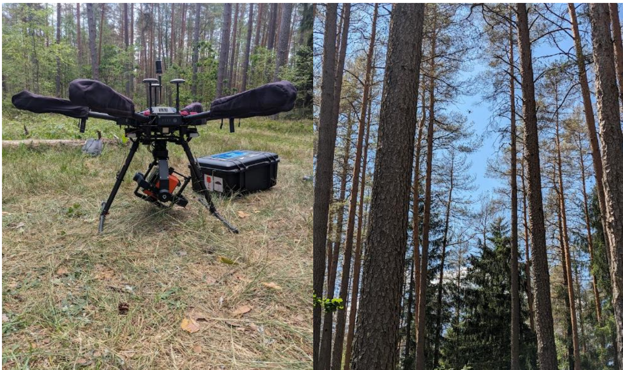
Figure 32: The UAV (multi-rotor) used for tree health inspections, mounted with a hyperspectral camera.
