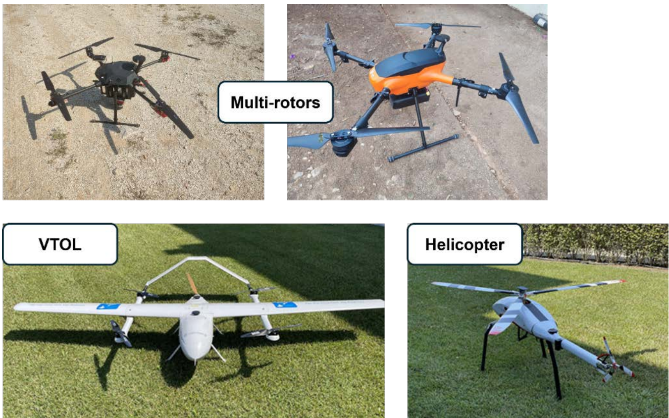
Figure 48: Three different UAV types for the implementation of rural logistics, depending on the type and size of the cargo, as well as to the distance of the delivery point.
