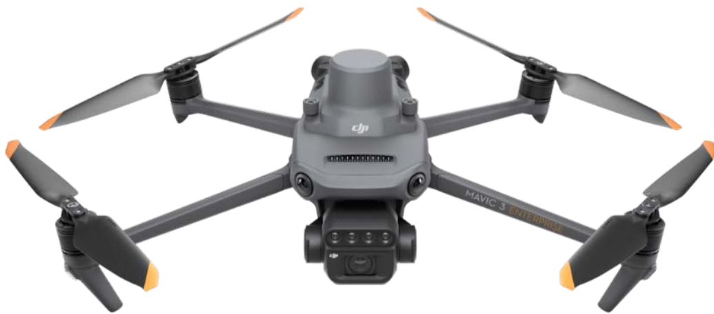
Figure 10: UAV platform (DJI Mavic 3M) used for crop monitoring implementation within UC1 of the ICAERUS project.
