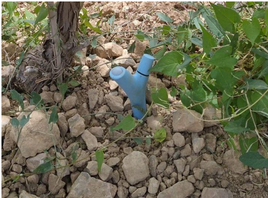
Figure 11: Weather sensor used for crop monitoring implementation within UC1 of the ICAERUS project.
