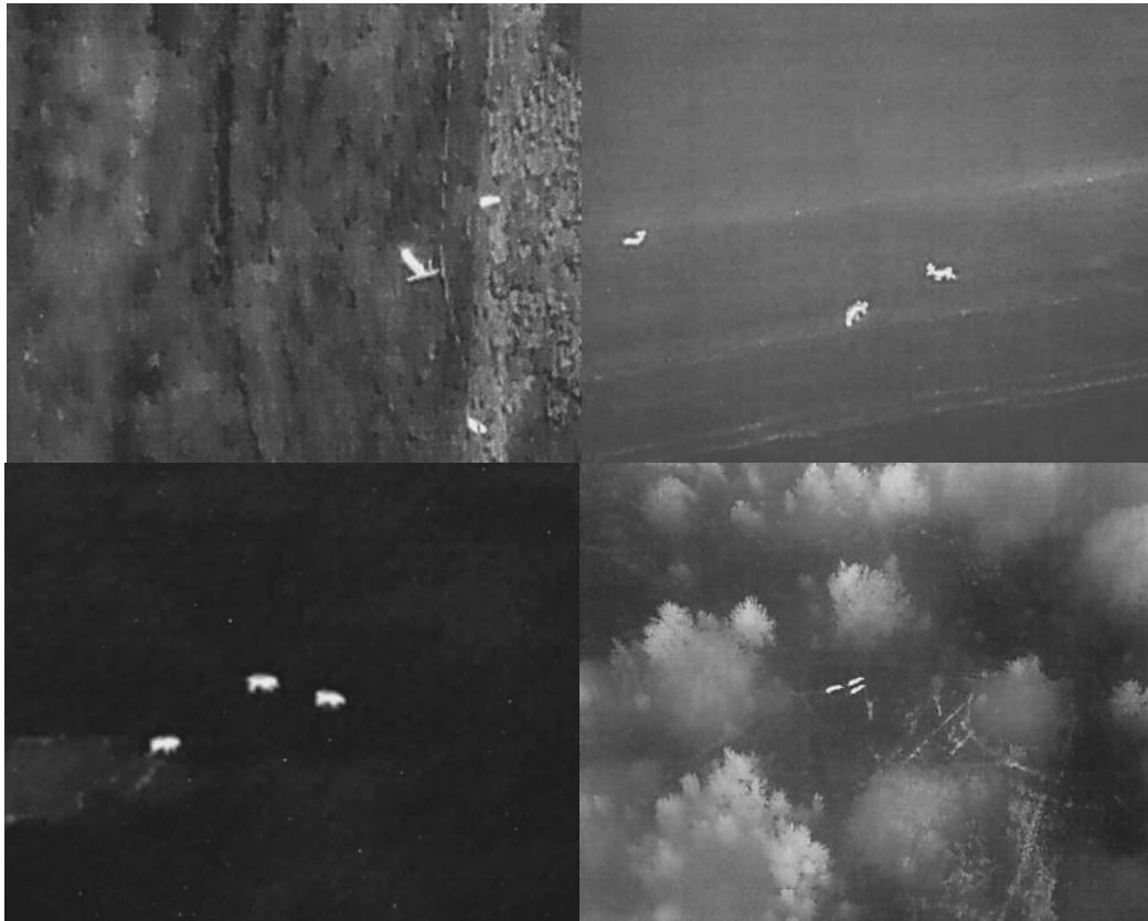
Figure 38: Example of animal detection from hyperspectral images that were captured during UAV operations. Different types of animals can be distinguished from the images.
