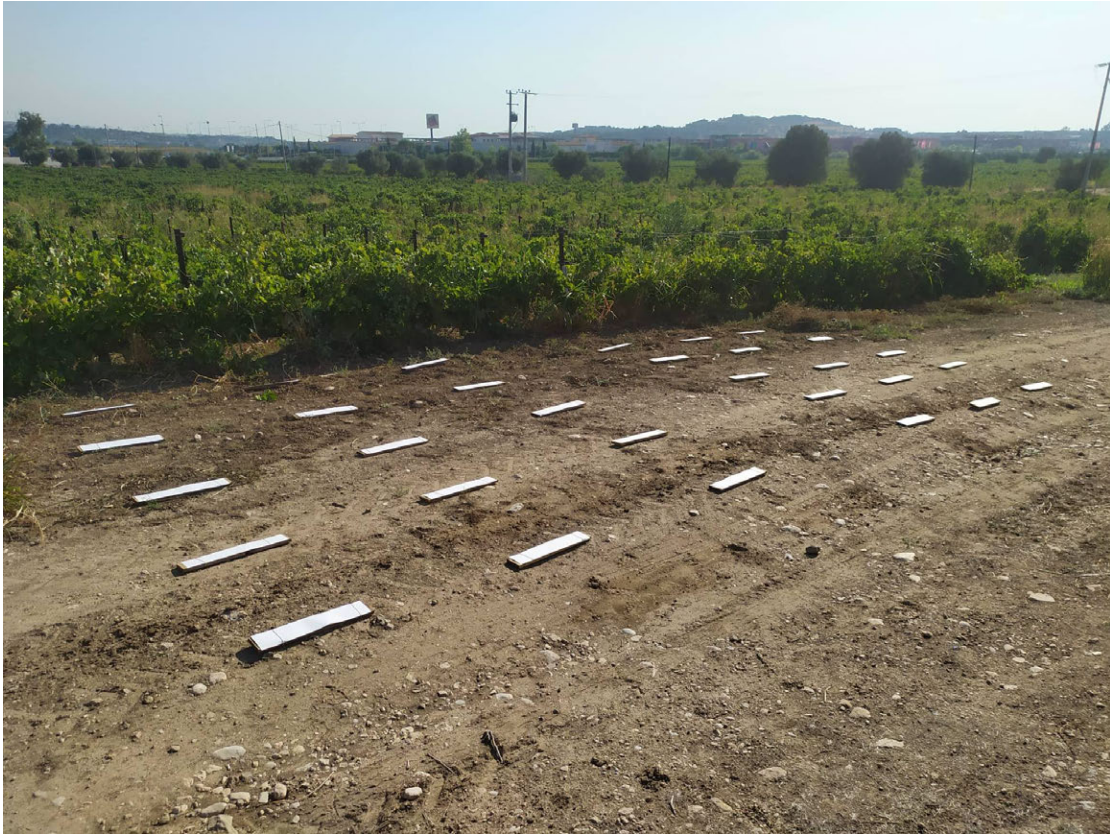
Figure 14: The filter paper collectors used at the first 5 sampling distances (1 to 5 m from the last vine row)
